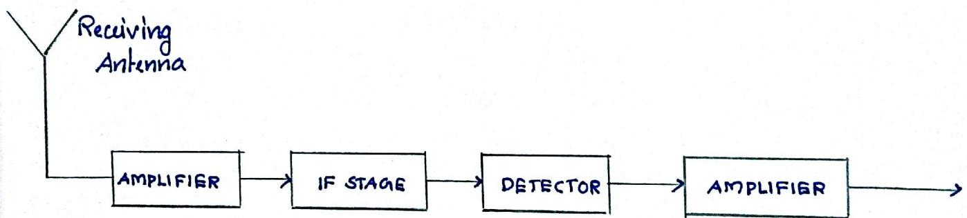
Detection is the process of recovering the modulating signal from the modulated carrier wave. Block diagram is shown in fig
